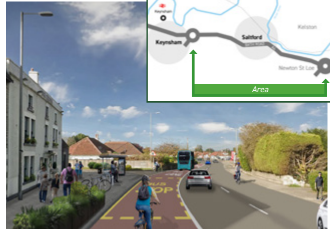
Short sections of bus lane are proposed in Saltford to prioritise buses in key locations
